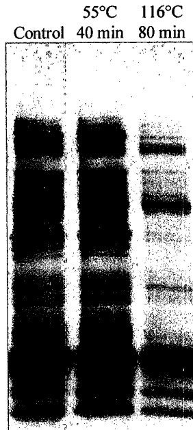
Figure 3: Comparison of albumin/globulin protein extracts of Hereward from control and selected heat treatments.
